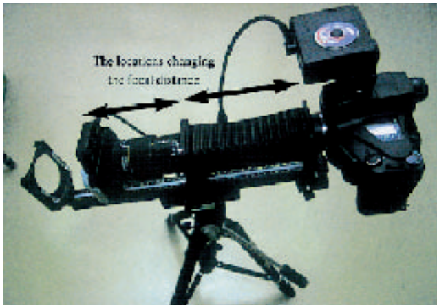
Fig. 1 The instrument for a shot and locations changing a focal distance.
